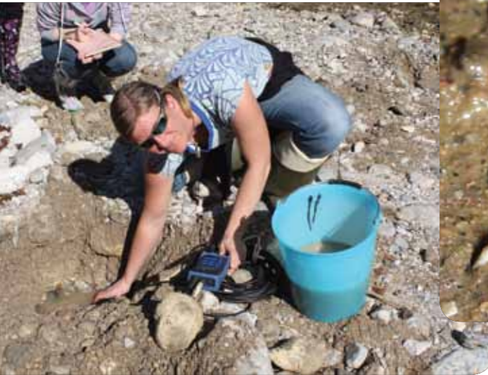
Meritve kisika v plitvem hiporeiku reke Soče pri Bovcu Measurements of oxygen concentrations in the shallow hyporheic zone of the Soča River near Bovec
