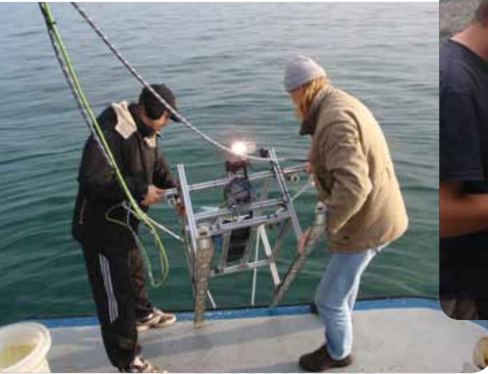
Spuščanje kamere na "podvodnih saneh" Video camera mounted on underwater skis
