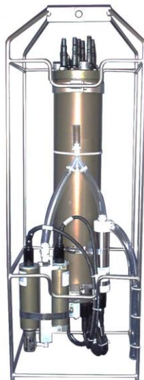
Slika 2: CTD sistem Sea-Bird Scientific SBE911
