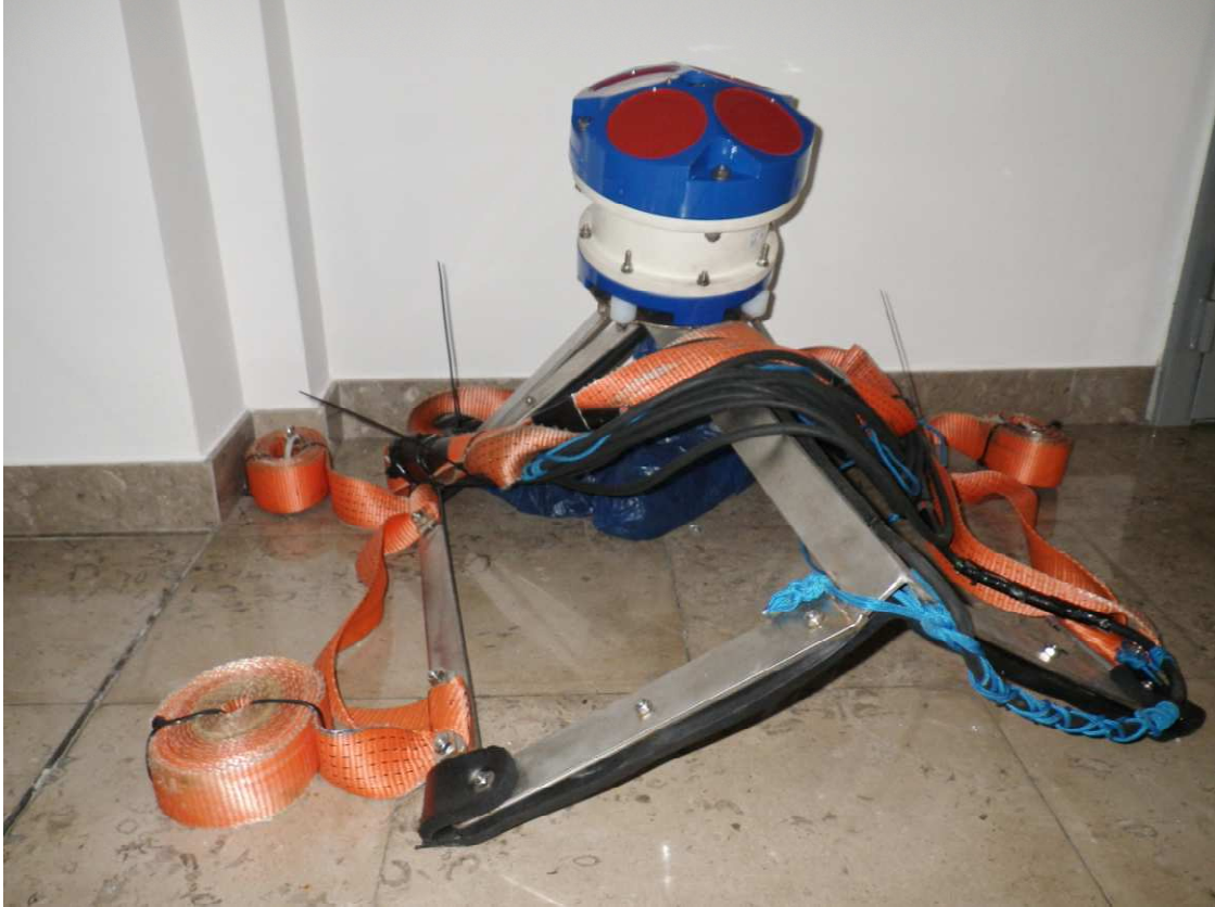
Figure 3: RD600 kHz workhorse, mounted on a frame for the installation on the vessel.
